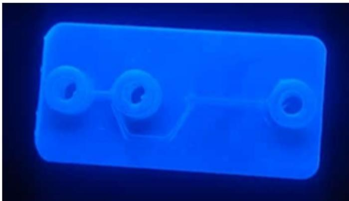
Figure 3. Microfluidic device in a UV Curing Oven
