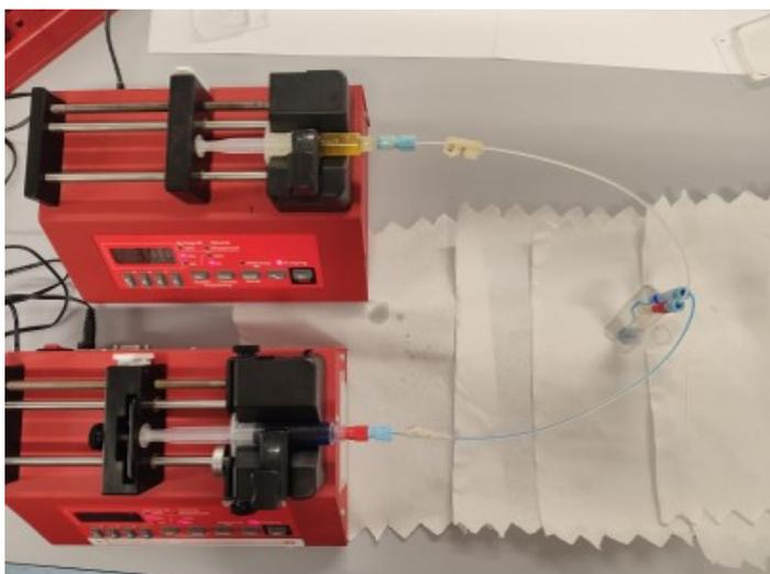
Figure 4. Droplet generation system with syringe pumps
