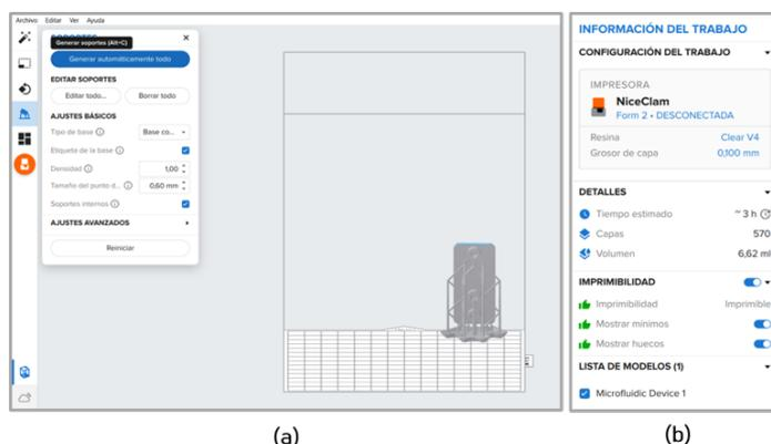
Figure 2. 3D Printing process configuration in Preform: a) Support structures generation. b) Printing parameters
