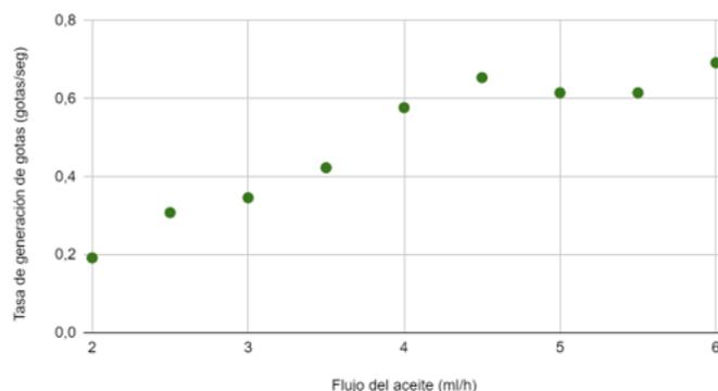
Figure 5. Droplet generation rate as a function of continuous phase (oil) flow
